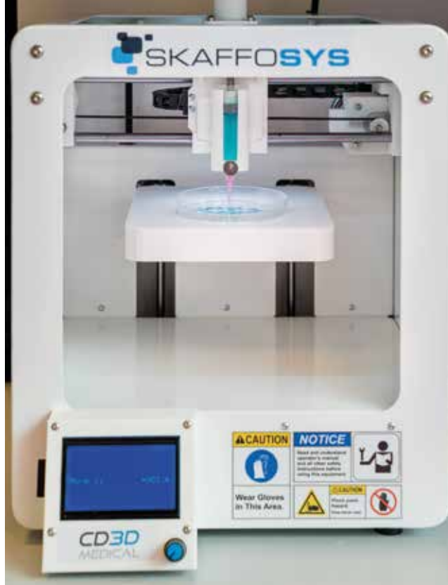
Bioprinting process – building three-dimensional structure from biocompatible hydrogel material
