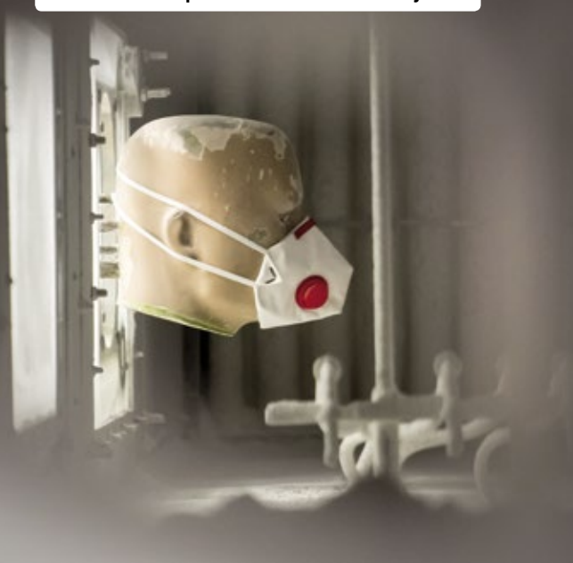
Clogging test for filtering facepiece respirator with time-dependent antimicrobial activity
